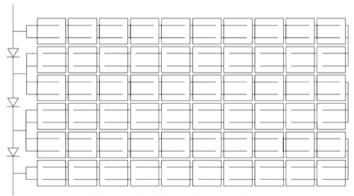
Example of Electrical Circuitry of Cells and Bypass Diodes
